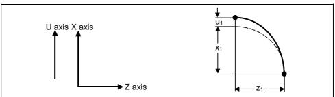
G18 G03 Xx<sub>1</sub> Uu<sub>1</sub> Zz<sub>1</sub> li1 Kk<sub>1</sub> Ff<sub>1</sub> ; ZX plane arc, U axis linear
